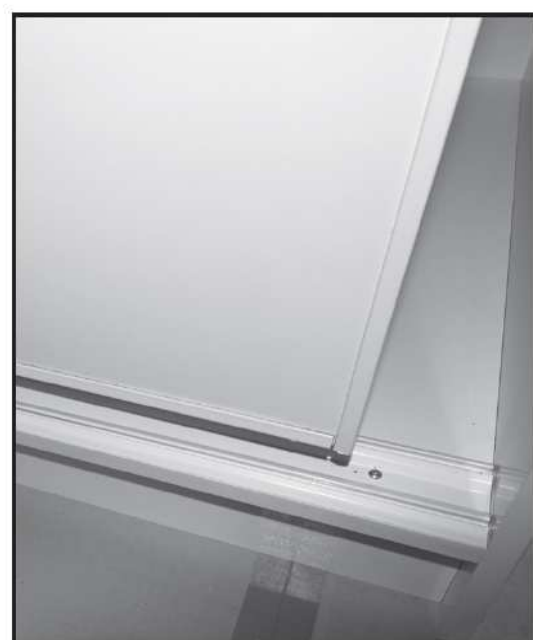
Step 4 - Lift the door and position its bottom wheels into their corresponding guide on the wardrobe floor.
